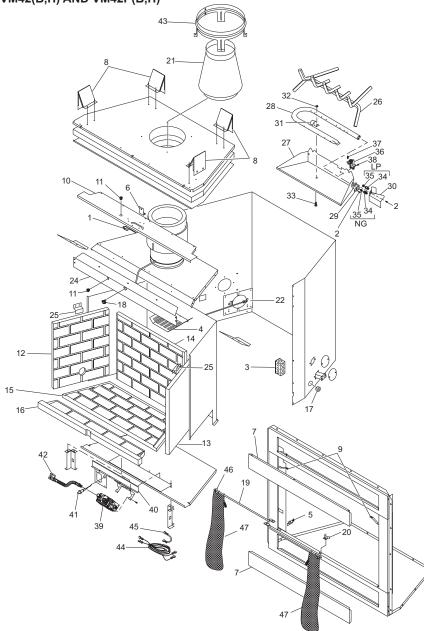
This list contains replaceable parts used in your heater. When ordering parts, follow the instructions listed under <u>Replacement Parts</u> on page 22 of this manual.
